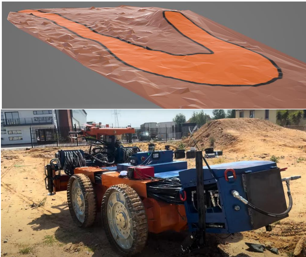
Figure 24 Top) Coarse 3D rendering of CMTI's test site. This render was generated from LiDAR scans that were accumulated during experimentation. Drivable portions are shown in orange with a dark outline. Notice the ramp area at the top of the image. Bottom) Real view of the CMTI surface test site.
